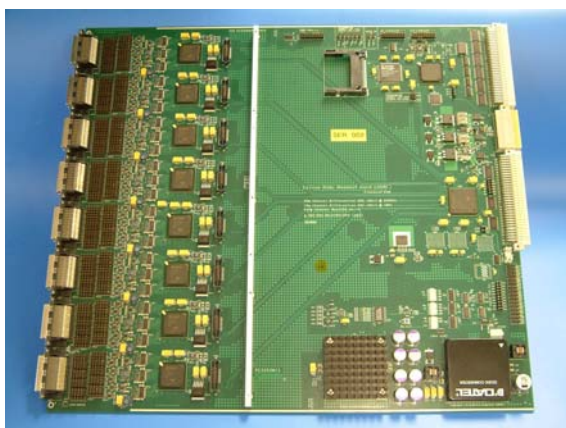
Figure 8-9 CALICE readout card CRC.
