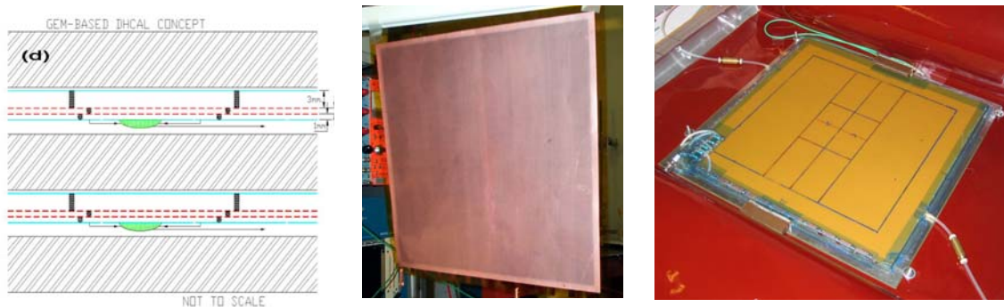
Figure 7-4 Left: GEM-DHCAL scheme. Middle: 30x30cm² foil. Right: Completed GEM chamber
