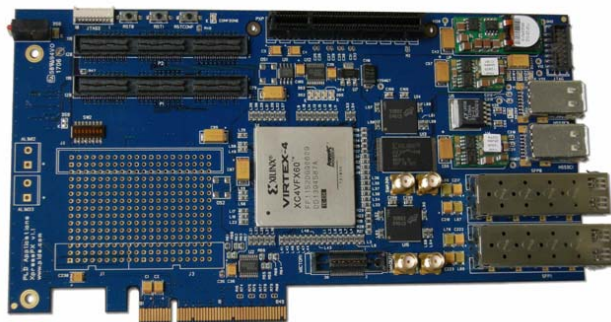
Figure 9-2: Physical DAQ card bought from PLD applications.
