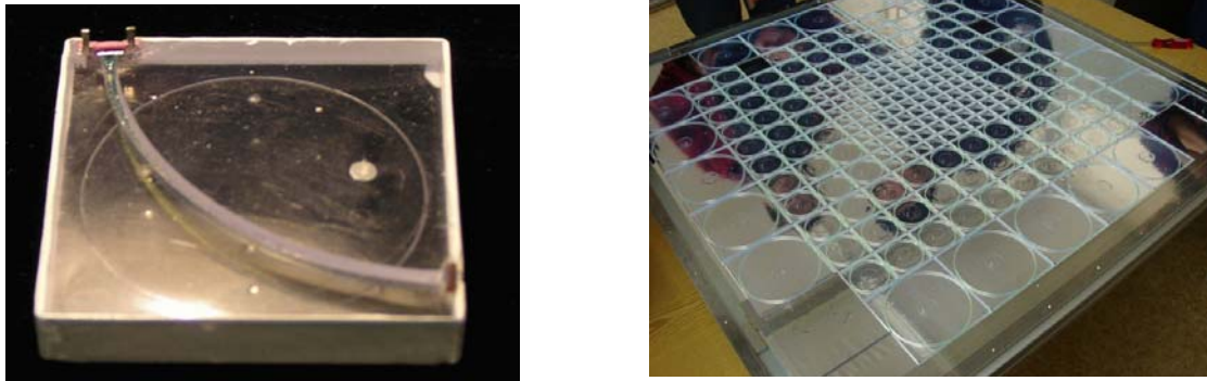
Figure 5-2 Left: Scintillator tile ( 3 \times 3 \text{ cm}^2 ) with SiPM. Right: Scintillator tile layer.
